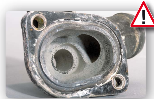
casing covered in lime scale
